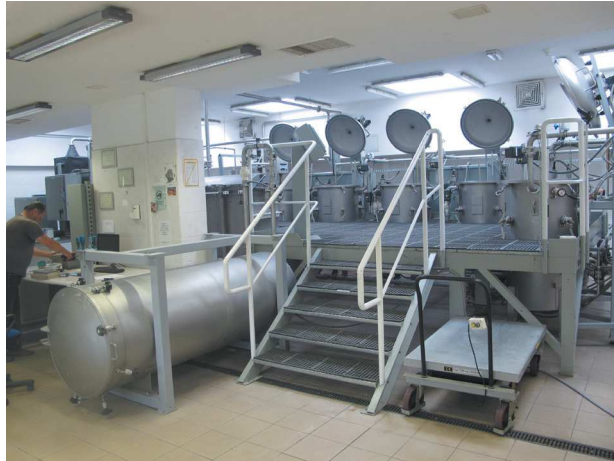
The Bookkeeper treatment. The deacidifying agent is MgO (as a fine powder) suspended in perfluoroheptane. Since no water is used in the process, it allows to treat books without dismantling them. The books attached to plastic frames are treated in the vertical reactors (photo: Bartosz Szymański).
