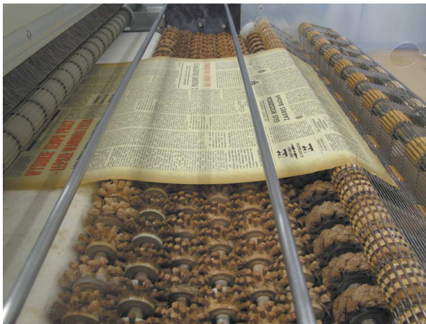
Neschen C-900 treatment. The objects on a steel band are submerged in a deacidifying solution containing alkaline agent ( Mg(HCO_3)_2 ), methyl-hydroxyethyl-cellulose and fixing agents: Mesitol NBS and Rewon EL. It is a machine version of the Bückeburg process (photo: Bartosz Szymański).
