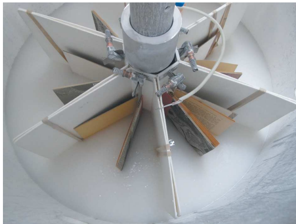
The Bookkeeper installation of the National Library. In addition to the vertical reactors there are also two horizontal reactors for treatment of single sheets or heavily damaged or fragile objects. The whole process is fully automated and computer controlled (photo: Bartosz Szymański).
