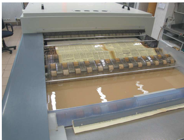
Neschen C-900 treatment. After the bath in the deacidifying solution the sheets are transported to the air drying channel of the C-900 unit. At the end of the process the paper should be humid enough to allow flattening under pressure between cardboards (photo: Bartosz Szymański).
